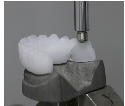
Figure 6. Typical failure mode of a milled PMMA interim prosthesis on the posterior region during the application of the load.
