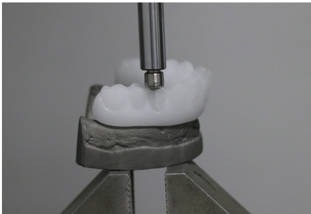
Figure 8. Predominance of a typical failure mode of a milled PMMA interim prosthesis on the premolar region during the application of the load.
