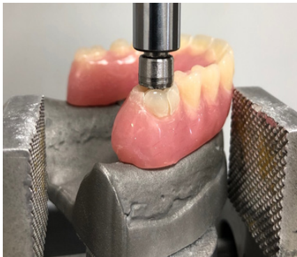
Figure 4. Typical failure mode of a conventional PMMA interim prosthesis on the posterior region.
