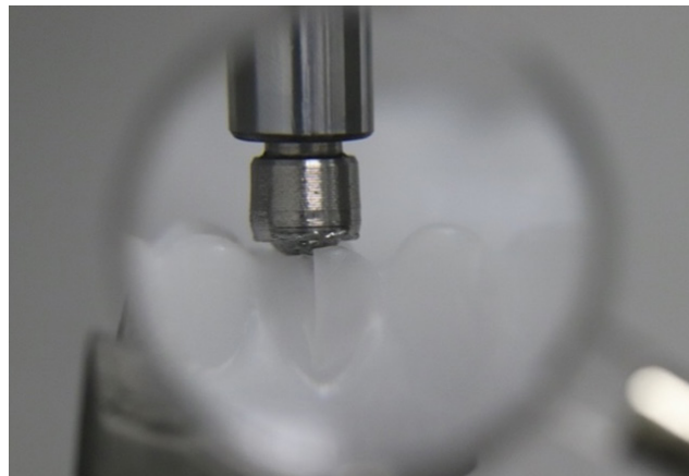
Figure 9. Typical failure mode of a milled PMMA interim prosthesis on the anterior region after the application of the load seen under a magnifier.
