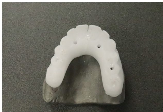
Figure 11. Typical failure mode of a milled PMMA interim prosthesis on the anterior region after the application of the load.
