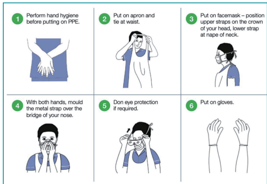
Fig. 2: Illustration for the order of putting on personal protective equipment (PPE). (Public Health England gateway [21]).
