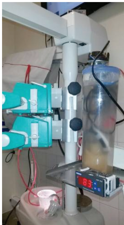
Fig. 4: The water heater with the 3 m tube inside it and the temperature of the water is 83 °C.
