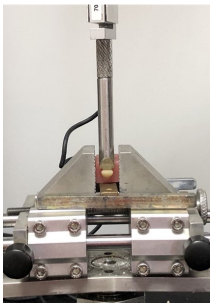
Figure 1. Sample in the universal testing machine.
