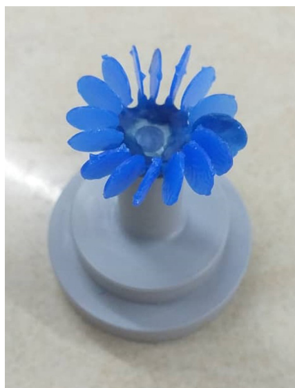
Figure 2. Wax discs and their preparation for LS2 injection
