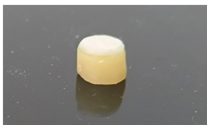
Figure 3. Ceramic disc after bonding to resin base
