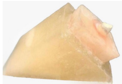
Figure 3. Custom-made jig to fix specimen at 45 degrees angle
